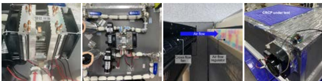
(a) TEM (b) Hydronic circuit (c) Air flow supply (d) Chamber
